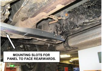
8. Mount and secure bracket to the 4 bolts on vehicle cross member. *Tighten cross member bolts to specified torque.*
