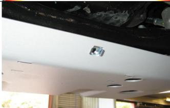
3. Fit M8 cage nut to centre point on rear of panel.
