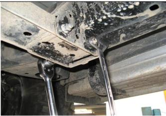
7. Before fitting transmission panel the mounting bracket needs to be attached to the rear of cross member. As shown in photo remove mounting nuts from gearbox cross member. NOTE: If you have side rails fitted it may be required to orientate bolts so they are placed in from front to back.
