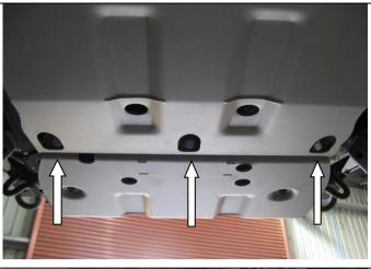
6. Secure front of sump panel to front panel using 3 x M8 bolts, spring washers and flat washer supplied, *tighten to specified torque*. Use M8 flange nuts on outer holes.
