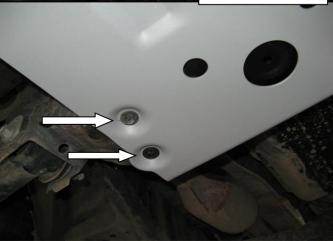
5. Fitting sump panel. As per step 2 fit an M8 cage nut to centre rear of panel. Lift panel into position and secure to cross member using original M8 bolts as shown. Leave finger tight.
