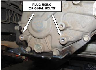
11. It is advised to have a drip-tray handy for this procedure even though it may not be needed. Remove original transfer case shield and retain bolts. Remove four lower case bolts and retain. Fit transfer panel as shown using original bolts. Fit remaining bolts into original mount positions at rear.
