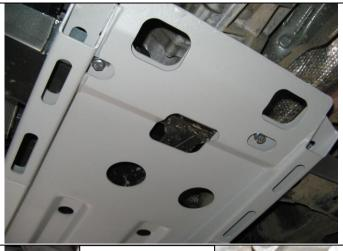
Secure panel to mounting bracket using 2 x M8 bolts, spring washers, flat washers AND flange nuts supplied. When satisfied tighten all bolts to specified torque.
