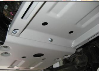
9. Lift transmission panel into place and secure to sump panel using 3 x M8 bolts, spring washers and flat washers supplied. Leave finger tight.
