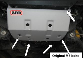
4. Mount front panel to vehicle using original bolts and positions. If fitted with an ARB bar place panel on top side of bullbar stone shield. Leave bolts finger tight.
